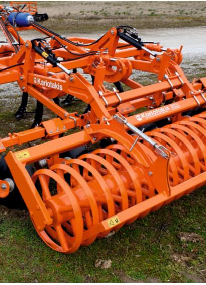
All rear rollers are Hydraulically Adjusted
