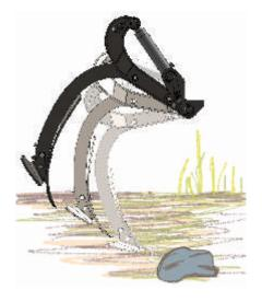
The improved Non Stop arm system at MasterMix allows an exact point control in the desired working depth – even in heavy soils and large working depths.
